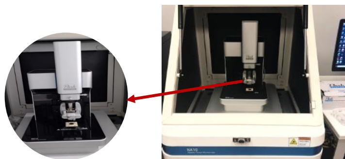
Figure 2. Atomic Force Microscopy NX10 Park System
