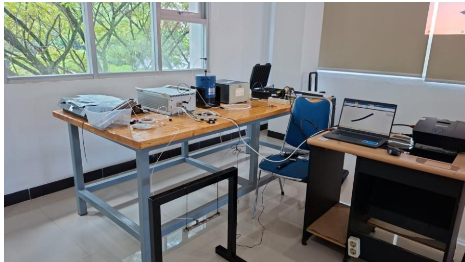
Figure 2. Experimental modal analysis setup with impact hammer, accelerometer, data acquisition system, and modal analysis software
