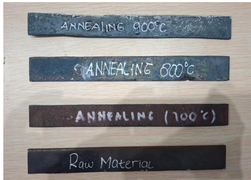
Figure 1. SS400 specimen conditions used in the experimental modal analysis
