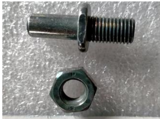
Figure 1. Failed rear-sprocket mounting (nap gear) bolt and nut used as the failure-analysis specimen.
