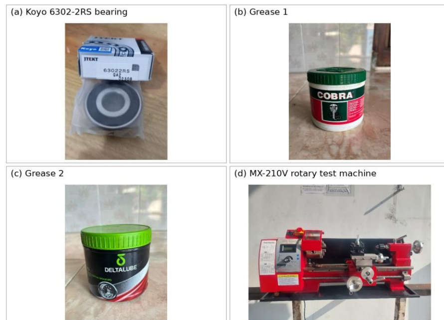
Figure 1. Main specimens and equipment: (a) Koyo/JTEKT 6302-2RS bearing, (b) Cobra ® Chassis Grease Green No. 3, (c) Deltalube ® 056 General Purpose Grease EP 2, and (d) MX-210V rotary test machine.
